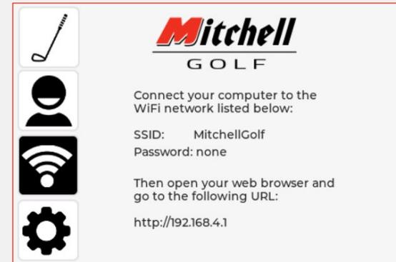
The digital display can project loft and lie measurements to a browser on a larger screen via Wi-Fi.
